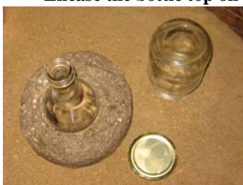
Mount the mounted bottle top over the vent hole and cover with a jam jar
