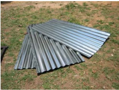
Three sheets are used each 1.5m long. These are cut from 3m sheets. The three sheets are fastened to the wooden frame with small nails with large heads. Each sheet overlaps the one next to it.
