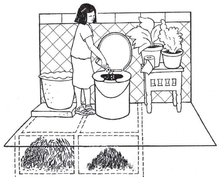
Figure 1: Double-vault urine-diverting dry eco-toilet in use in China, Vietnam, Mexico, and India
