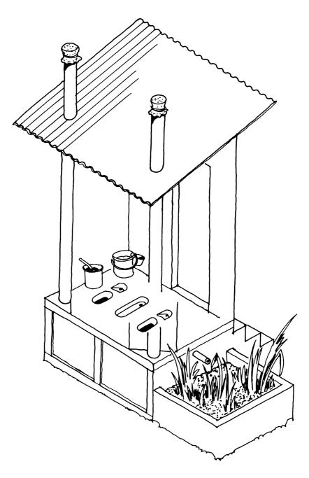
**Fig 3.20** The Kerala double-vault toilet. Over each vault there is a drop hole for faeces and a funnel for urine. Between the two vaults is a trough over which anal cleaning is performed. The water used for anal cleaning and the urine flow into the evapo-transpiration bed planted with bitter gourd, plantain or Cana indicus.
