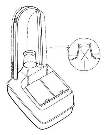
Figure 3.16 The 'Sirdo Seco' double-vault, solar-heated composting toilet in Mexico. The whole toilet, including the superstructure, is made of fibreglass.
