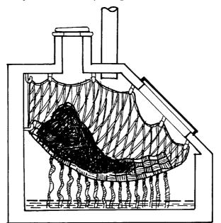
Figure 3.18 The CCD composting toilet, designed for the extremely humid climate of the South Pacific. It has a 'false floor' made of a fishing net to separate liquids and solids, and wicks from old clothing to increase evaporation.
