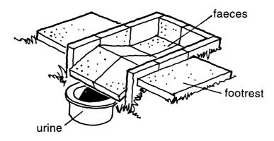
**Figure 4.5** A traditional toilet with urine diversion in China. Urine is collected in a jar and used as a liquid fertilizer for vegetables. (Faeces are scooped up daily and taken to a compost pile.)
