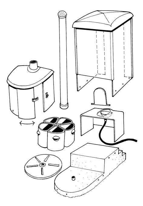
Figure 5.5 Exploded view of the toilet in Figure 5.4.
