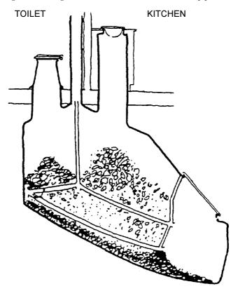
**Figure 3.13** The 'Clivus' Multrum composting toilet from Sweden placed in the basement of a house. This model has a separate chute from the kitchen for food left-overs etc. Perforated pipes bring air into the centre of the compost pile.
