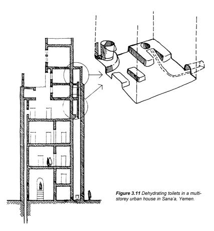
Anal cleaning takes place on a pair of square stones next to the squatting slab. The water used for anal cleaning as well as bath water is drained in the same way as the urine. No liquids are thus led into the long drop shaft or the vault below. As Sana'a has a hot, dry climate, the faeces quickly dry out<sup>6</sup>.
