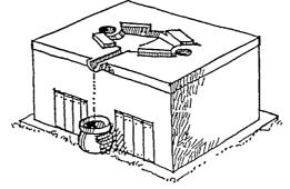
**Figure 3.2** The processing chambers of Figure 3.1 provided with a squatting slab for urine diversion, a pot for collecting urine and lids for the two openings for removal of dehydrated material. The drop hole not in use is closed with a stone and sealed with mud or mortar.
