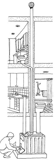
**Figure 4.3** A Clivus Multrum system in a multi-storey building. The lower bathroom has a dry toilet with a chute straight down to the processing chamber. The kitchen has a another chute for organic household refuse. The upper bathroom has a minimum-flush toilet.
