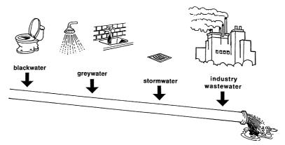
**Figure 1.1** In a flush-and-discharge system a relatively small amount of dangerous material – human faeces – is allowed to pollute a huge amount of water. In most cases the resulting sewage is discharged completely untreated into surface waters.
