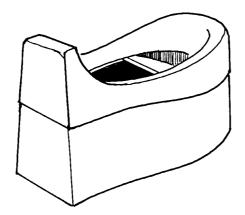
Figure 2.5 Seat riser with urine diversion, made of fibreglass. The pan was developed by the Sanres funded project in Mexico in 1994.
