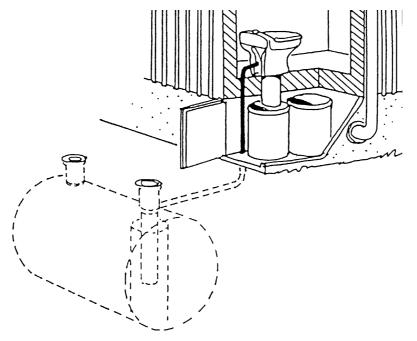
**Figure 3.6** A dehydrating toilet of type 'WM Ekologen, type ES' installed inside a house in Sweden. Faeces and toilet paper are dropped into a large bucket. Urine is piped into an underground storage tank.
