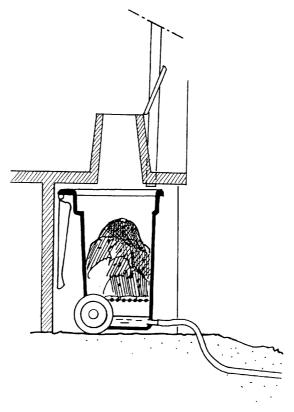
*Figure 3.17* A composting toilet with liquid separation. The processing chamber is a standard wheeled plastic refuse bin modified to drain away excess liquid.
