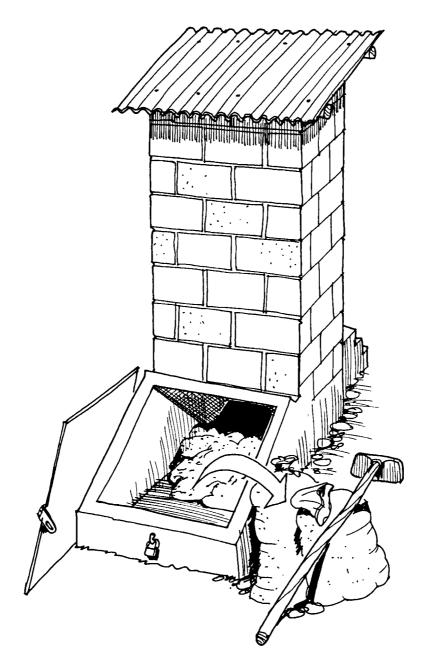
**Figure 4.7** A single-vault dehydrating toilet in El Salvador. The pile building up below the toilet seat is periodically shifted to the processing chamber under the solar heater. When this space is full the material is taken out and placed in bags for further storage until ready for use as fertilizer.
