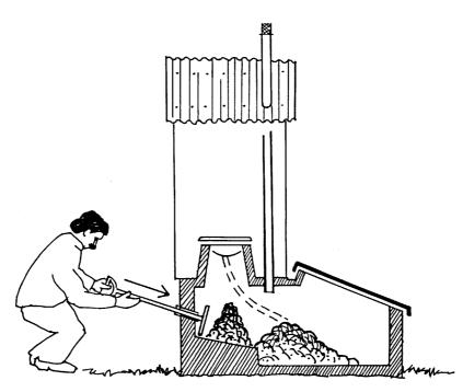
Figure 3.9 A few times a month a fixed pusher is used to shift the pile of faeces and ash from below the toilet seat into the solar heated processing chamber.
