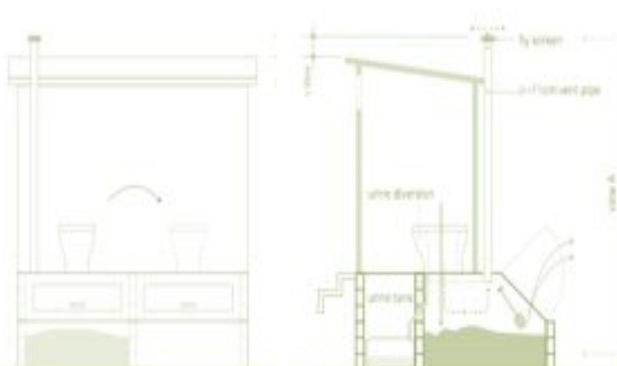
schematic of a 2-chamber UDDT
