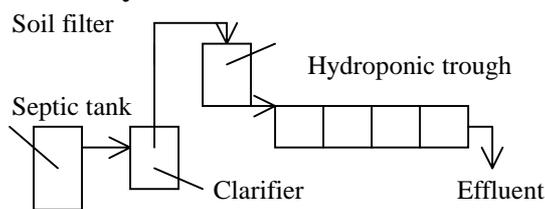
Fig. 1 Diagram of filter and hydroponic system
