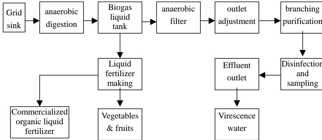
The technique consumes no energy which means low operating costs. It can recover biogas with satisfactory treatment results. The treated effluent can reach the third or second issued discharge standard and it can be used as virescence water around the toilets. Besides, efficient organic liquid fertilizer can be developed from the biogas fluid coming from biogas fluid tank. Such fertilizer is handy to use with sanitation and perfect fertility.
