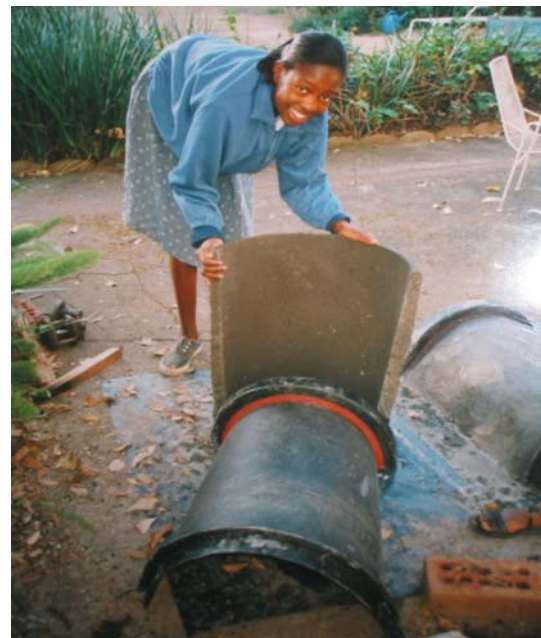
Making the larger 80 litre split cement jar using a plastic dustbin as a mould.
