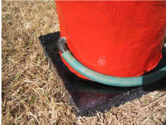
The pedestal can be made more attractive by coating with enamel paint once the concrete is completely cured and dry. Once dry it can be mounted into the toilet.
