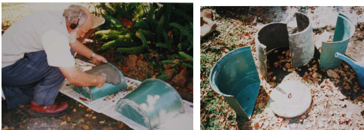
Plastering the two shells of the 30 litre split cement jar on a mould made from a 30 litre plastic bucket. After a few days of curing the two cement shells can be separated from the mould.
