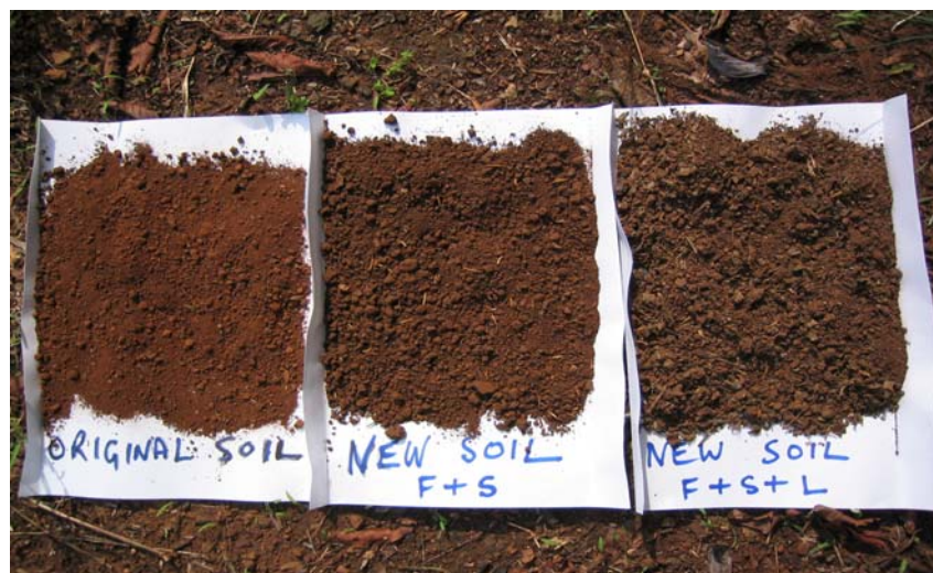
Samples of original soil (left), and “new soil” made from faeces and soil (centre) and from faeces, soil and leaves (right)
