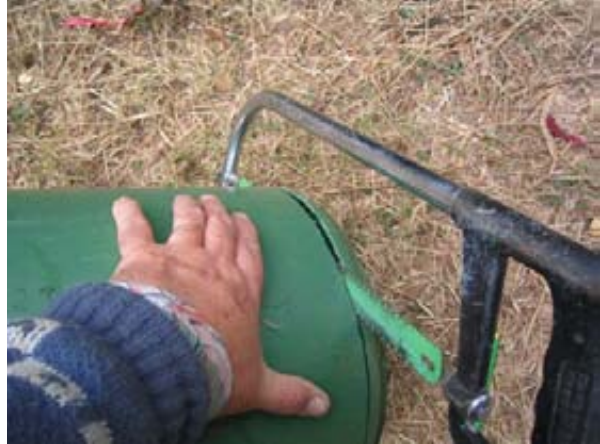
The material requirements are a 20 litre plastic bucket, a 20mm polyethylene bend, a plastic toilet seat and cement, sand and wire. First the base is sawn off the bucket squarely.
