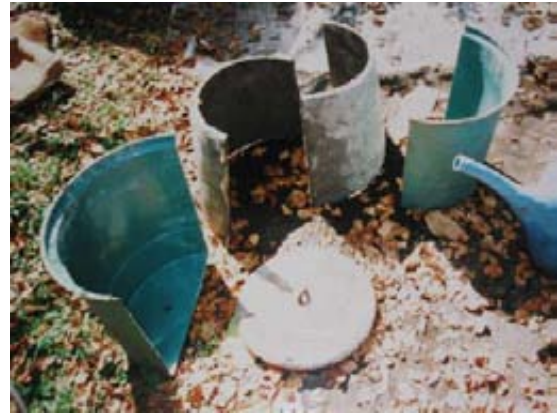
Plastering the two shells of the 30 litre split cement jar on a mould made from a 30 litre plastic bucket. After a few days of curing the two cement shells can be separated from the mould.
