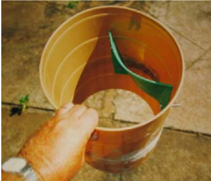
In this method a piece of plastic from a bucket is bolted to the side wall of the larger chute bucket to make the urine diverter. At the base of the diverter a polyethylene pipe is fitted in place with epoxy putty. Urine passes down the diverter, through the pipe into the urine storage vessel. This plastic unit is then built up in cement and a seat is fitted as described earlier.
