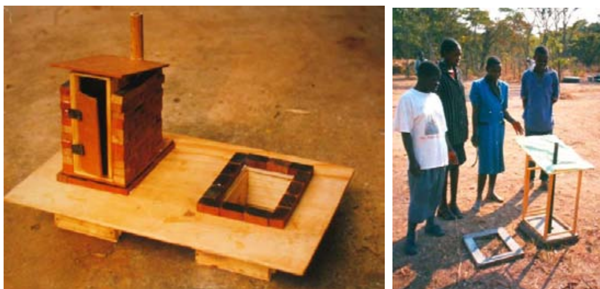
Two models used to teach people about the Fossa alterna . Models are valuable teaching aids.
