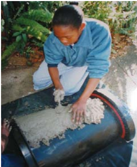
Making the larger 80 litre split cement jar using a plastic dustbin as a mould.
