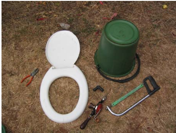
The material requirements are a 20 litre plastic bucket, a 20mm polyethylene bend, a plastic toilet seat and cement, sand and wire. First the base is sawn off the bucket squarely.
