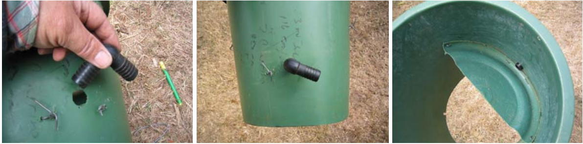
A hole is drilled through the bucket wall just above the base of the urine diverter. The 20mm polyethylene bend is fitted through the hole as shown. It is placed at the angle shown above.
