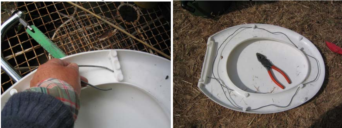
The toilet seat is now prepared. Using a hot wire, holes are drilled through the plastic ribs which support the seat. These allow a wire to be threaded in a loop under the seat.
