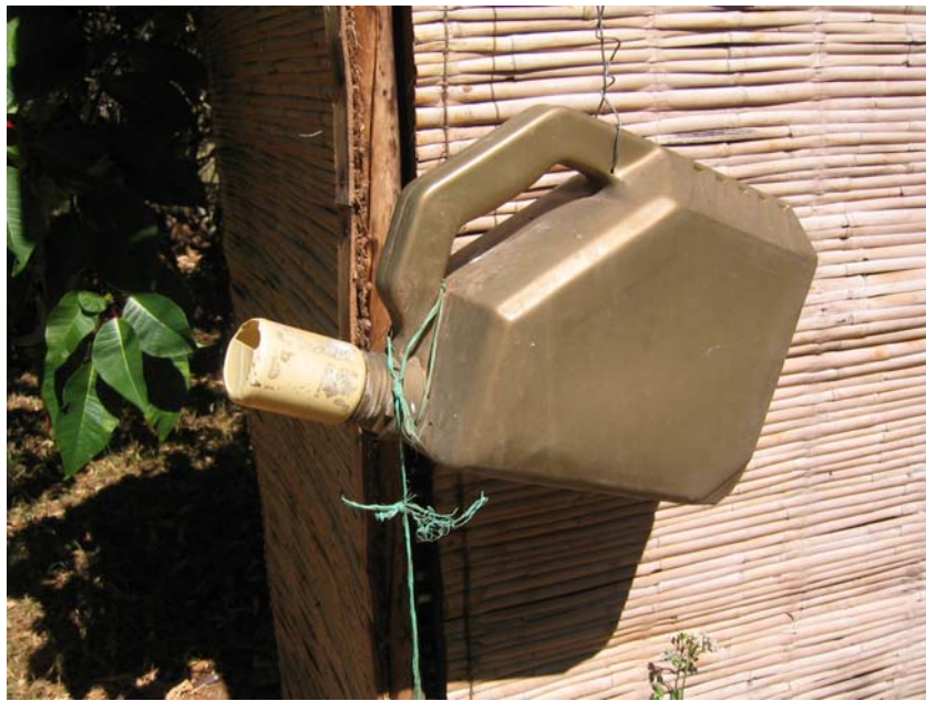
Hand washing device made from an old 5 litre oil container and pill bottle
