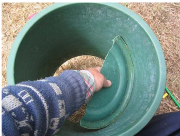
The half base is fitted within the bucket about half way up the walls at an angle. It is secured in place by drilling small holes through cut base and bucket walls and passing wire through and tightening.
