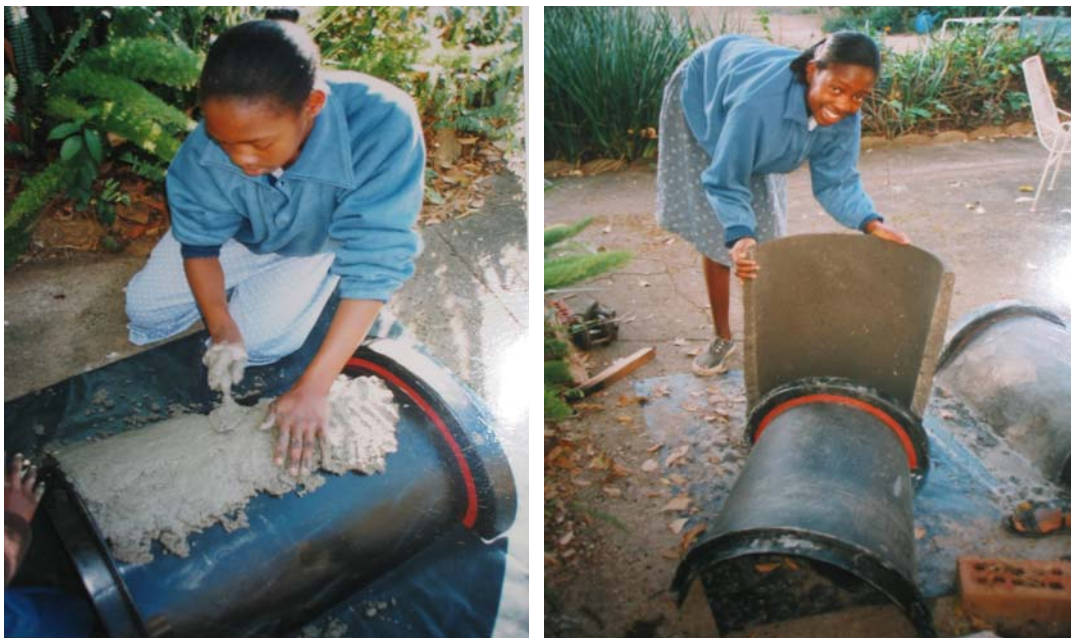
Making the larger 80 litre split cement jar using a plastic dustbin as a mould.
