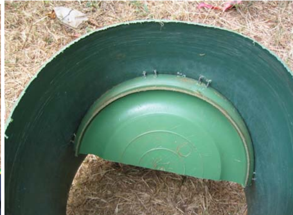
The half base is fitted within the bucket about half way up the walls at an angle. It is secured in place by drilling small holes through cut base and bucket walls and passing wire through and tightening.
