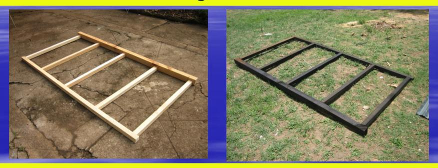
The wooden frame is made with 7 pieces of softwood. Most are standard brandering (38mm X 38mm). The front long timber is 2m x 76mm x 50mm, the rear long timber is 2m x 38mm X 38mm, The 5 shorter pieces are 0.95m long. This arrangement gives a slight slope to the roof once the iron sheets are fitted. The timbers are nailed together with 100mm nails. The frame is treated with a mix of old engine oil and carbolinium.
