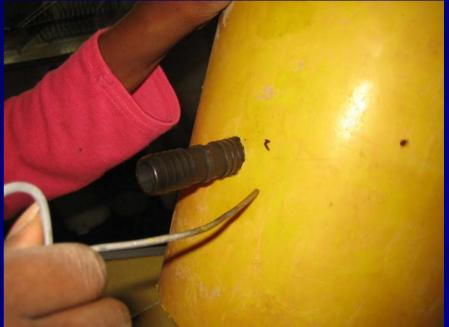
The position of the tin sheet is marked and a series of holes are made in the bucket with a hot wire.
