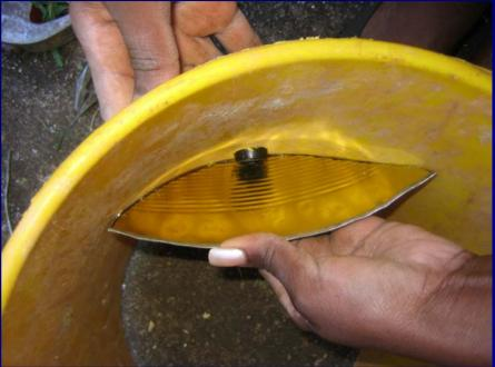
A tin sheet is cut from a opened up tin can, flattened and then cut into shape. This fits inside the bucket to form the urine diverter. It is held in place by wire.
