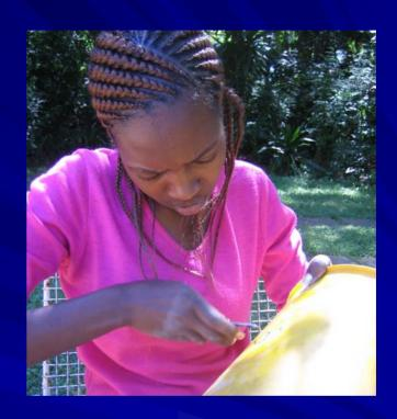
The base is cut off a 10 litre bucket. Carefully using a sharp knife a hole is made in the side wall of the bucket to take a 20mm poly-pipe fitting.
