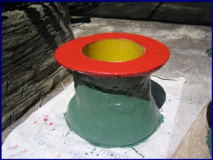
After this period it is allowed to dry out in the sun. The seat section is then filed and sanded down to make it smooth. It can then be coated with enamel paint. Bright colours are best!
