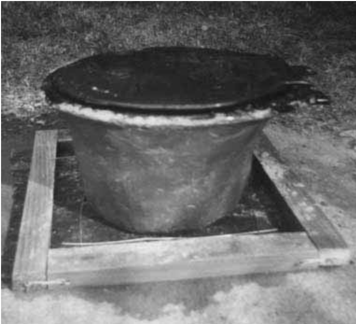
Figure 5-11: Completed pedestal placed in wooden mould
