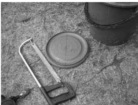
Figure 6-9: Marking the plastic base
