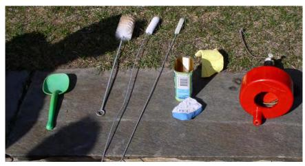
Figure 26. Cleansing tools for a urine-diverting toilet. Photo: Ebba af Petersens.
